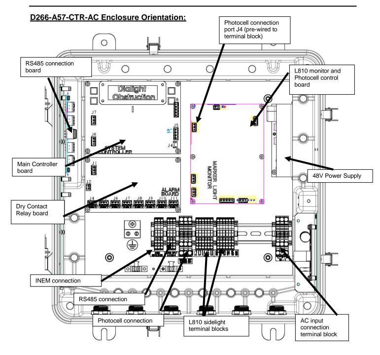
**NOTE:** Multiple grounding points are provided in the enclosure for protective and functional Earth/Ground connections.
